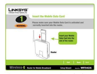
Figure 7-3: Insert Broadband Mobile Data Card Screen
